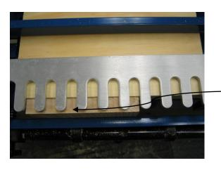
4. Secure this piece vertically on the left side of the jig so that it is centered on the template fingers. Ensure that its end is fully registered against the template. Set the left side stop against the edge of the test piece.
