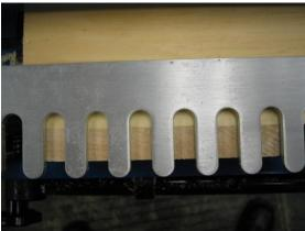
6. Install the ½" 8-deg cutter in the router, place the router on the finger template, and use the line made by the marking gauge to set the depth of cut.
