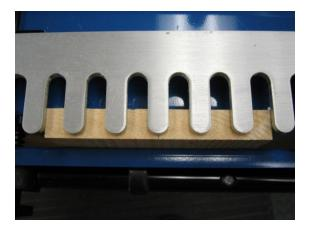
3. Clamp a test piece that corresponds to the drawer side vertically on the left hand side of the jig so that it is centered on the template fingers. To insure it is clamped squarely, its end must be fully registered on the template. Loosen the screws securing the vertical stop and adjust the stop to touch the edge of the workpiece.
