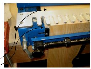
3. Prepare a test piece the same width and thickness as the dovetail stock. Use a marking gauge set to the stock thickness plus about 1/32" to scribe a line across the ends.
